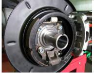
Our RPB054 Brake kit uses the common VT-VZ Commodore "Banksia" park brake system, a 286mm rotor and calipers.
