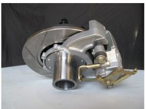
2 versions of this kit are available, both are based around Ford Falcon EA-ED Brake Calipers.
