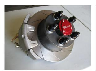
The Race Products RPB051 Brake kit has been designed to suit the 1500 Series Floating Hubs.
